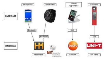
Figure 2 Hardware and Software for data collection
